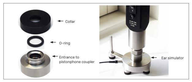
Fig. 6. Calibration using the pistonphone
